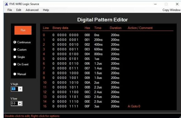
The Logic Source tool provides configuration, run control, and a pattern editor. Logic Source patterns can be saved and recalled later. Pattern files use a human readable CSV format which allows patterns to be generated in a spreadsheet or by user written programs.
