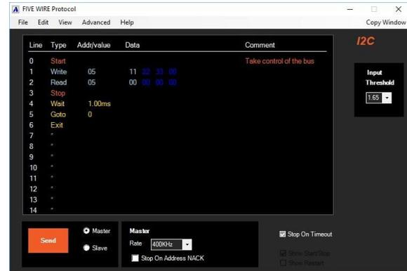
The I2C tool provides a transaction viewer and editor. When in master mode the user defines transactions that will be placed on the bus. In slave mode, captured transactions are displayed. Transactions can be saved to a human readable CSV file and reloaded at a later time.
