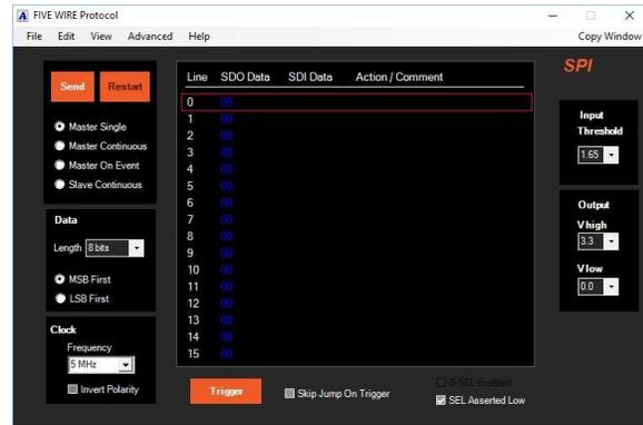
Commands and triggering can change the sequence of execution. When execution is stopped, the captured data can be inspected for proper operation.
